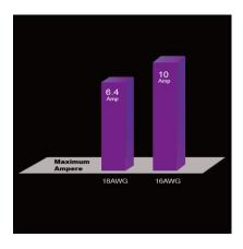
The thicker 16 AWG PCI-e cables allow for higher currents, because they have a higher heat tolerance, thereby improving efficiency and safety.
