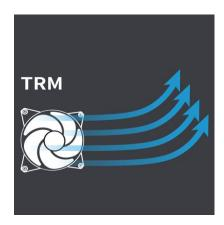
Thermal Regulation Mode (TRM) keeps the V Platinum quiet and stable by maintaining a constant fan speed up to 60% of the maximum load.
