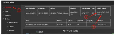
✓ Check the power, temperature, network status and fan status Click the Log in the menu as below.
